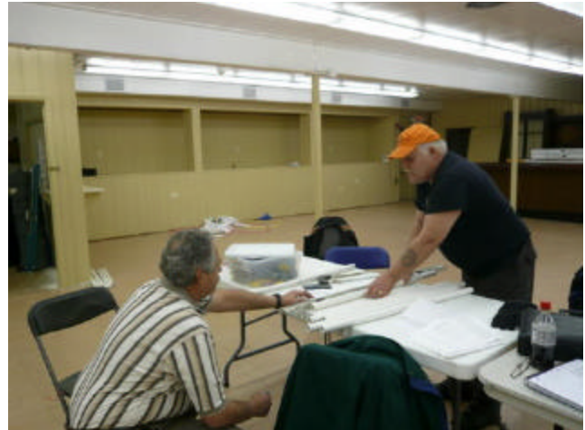
Fig 4. Max N9MYY and Carl N9KTL drawing the lines for the boom. It's important that these lines be as straight as possible to make sure the elements are all in the same plane.
