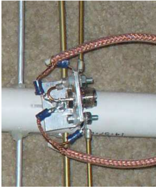
Fig. 5. A closer look at the bracket and coax balun of the 440 MHz antenna. The center conductor of the SO-239 is connected to one side of the T-match. The center conductor of the coax balun connects each side of the T-match together. If you build an array of similar antennas and stack them together for more gain, make sure to connect the center of the SO-239 to the same side of the T-match on each antenna to maintain a proper phase relationship. You can also see that each element is secured to the boom with hot glue.
