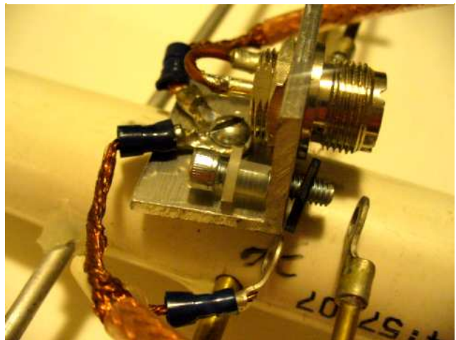
Fig 3. Another look at the bracket assembly. In this photo you can see the shield of the coax from the impedance matching section grounded to the bracket. Each side of the center conductor is attached to each side of the T-match.
