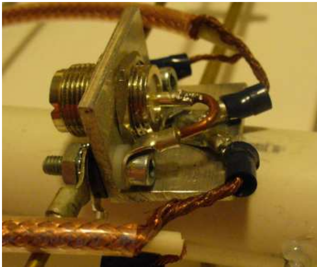
Fig. 1. The assembled bracket. Note the change to socket head screws. Even with the socket head screws, there still isn't much clearance to the bracket. You can also see in this photo that the center conductor of the SO-239 is connected to one side of the T-match by a very short section of solid 12-gauge wire. The coax balun connects to the other side of the T-match.
