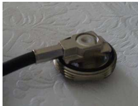
Fig. 1. The underside of Larsen's beefy NMO mount and the flowery print on the pad of the author's dining room table.
