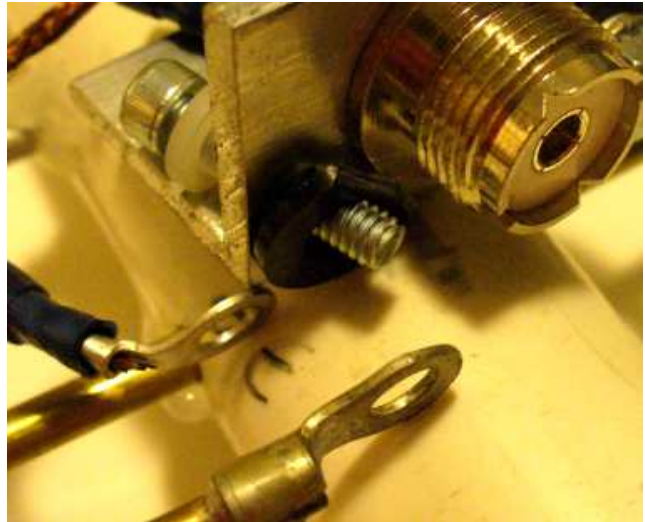
Fig. 2. Assembling the driven elements. The black nylon washer (note how the edge near the SO-239 is trimmed flat) and all the connections were made on the feedline side of the bracket, and the nylon bushing and the screw were fed through the hole from the other side.
