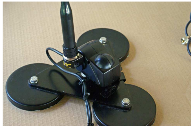
Fig 1. The antenna and motorized mount mounted to the DC Ace tri-mag mount.
