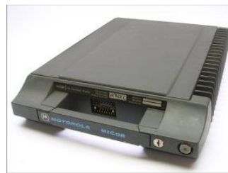
Fig 1. A Motorola Micor transceiver. This would typically be mounted in the trunk with a control head under the dash or in the center console. Mitreks and Syntors are very similar in appearance and size.
