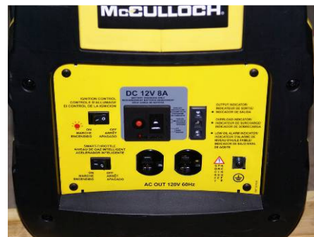
Fig 2. A close up of the outputs. The generator has 120 VAC as well as 12 VDC. The 120 VAC output is stable, but we haven't metered the 12 VDC side.
