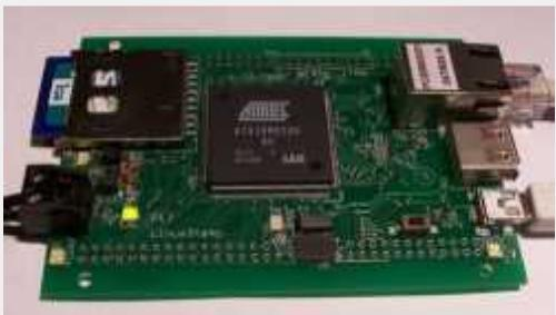
The Linuxstamp is an open source processor module based on the Atmel AT91RM9200 processor. All development can be done with the USB device port which is connected (via USB/serial chip) to the debug serial port on the Linuxstamp. The board's processor, a 180 MHz Atmel AT91RM9200 system-on-chip, integrates an ARM9 CPU core (with MMU) along with controllers for USB host and device ports, 10/100 Ethernet, MMC/SD card interface, sync/async serial ports, SPI (serial peripheral interface), and more.
