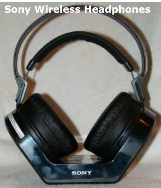
The headphones have a switch in the self adjusting head band that is activated when placed on your head, turning on the headset; this is so you can save the charge on the nickel-metal hydride AAA batteries when not in use and not placed in the charging cradle. The headphones also have a volume control. They are lightweight and comfortable to the point you forget you have them on ["What? I can't hear you, Marlene!" - Ed.]; mass is 300g (10.59 oz).
