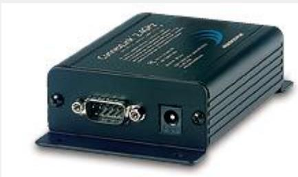
Our intrepid field reporter Steve KB9MWR has discovered this product from his QTH in the North Woods of Wisconsin. The AeroComm CL4490-1000 is a one watt 900 MHz Frequency Hopping Spread Spectrum (FHSS) RS-232 transceiver. The individual transceivers are available from Mouser Electronics for about \$110 each, though we recommend the starter pack that includes 2 transceivers for \$225.
