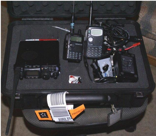
My original thought was to use my FT817ND and a Dual Band Elk LPA on 2 meters and 432 and a collapsible 6 meter Dipole all mounted on a camera tripod. The 223 station would then be my THF6 with it's "High Gain" rubber duck and then for 1296 my ICT91A again with a rubber duck. So that meant 5 watts on all bands except 1296 where I had a whopping 1.5 watts!
